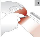
Cut the gel slightly longer than the length of the sleeve.
