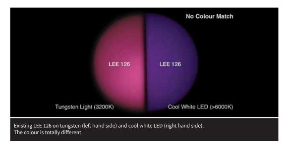
With cool white LED systems increasing in use, it became obvious that something had to be done, so the technicians at LEE Filters came up with a solution: the LED Filter range. These filters are designed to produce the same colour on a cool white LED (>6000K) as their tungsten-lighting equivalent. Try to think of them as a range of colour-corrected filters, as opposed to those that are colour temperature corrected.
