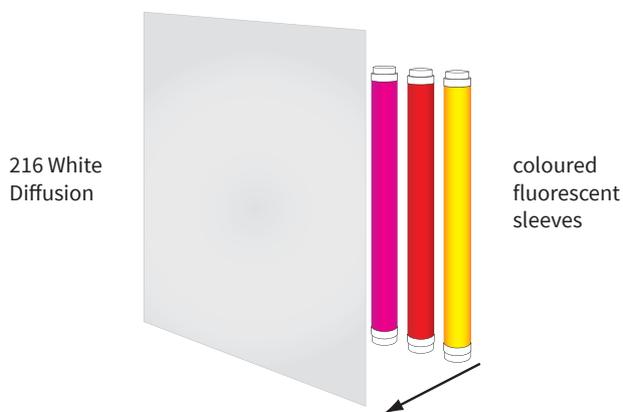
The distance between the diffusion and tubes determines the strength of the diffusion effect. The further apart, the stronger the effect; the closer together, the weaker the effect.
